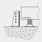
② Install the seismic stopper at a distance from the equipment where it does not come in contact during normal operation
